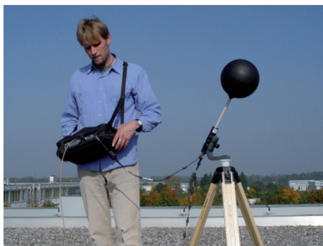
Measurement with 9102 Handheld Spectrum Analyzer and 9171 Isotropic Antenna
